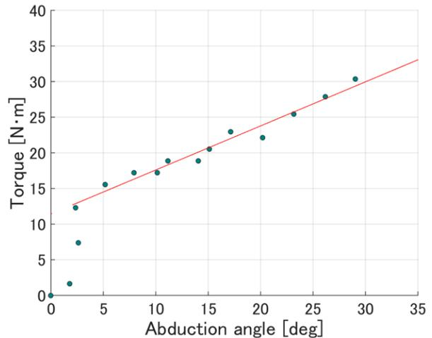
Fig. 3. The resistance torque of the exoskeleton against abduction angle
