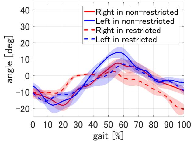
Fig. 9. Hip rotation angle in non-restricted and restricted cases including outer swing
