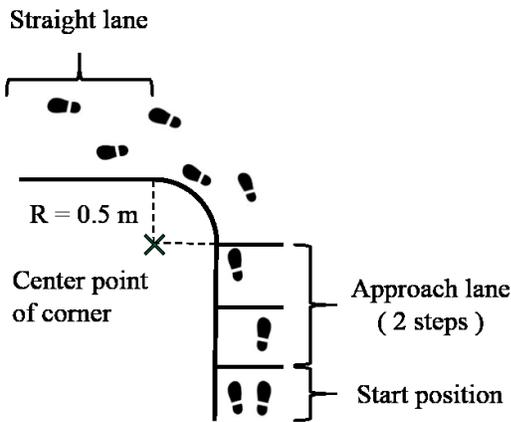
Fig. 1. The straight and curving path and the ideal foot steps
