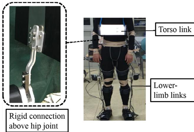
Fig. 2. The exoskeleton and its fixation part which restricts out-of-sagittal-plane motion
