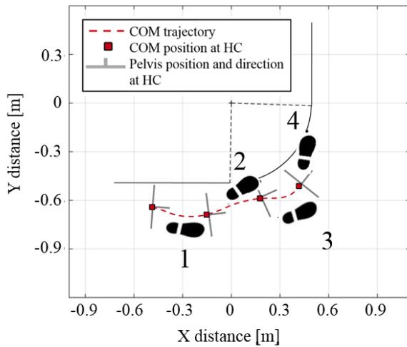
Fig. 6. The motion trajectory of an outer swing trial in the restricted condition
