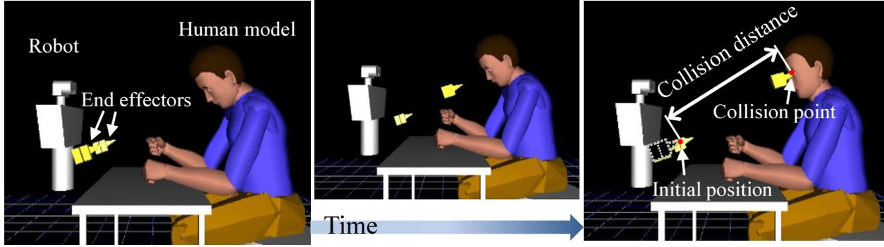
Fig. 4. A series of screen images in extrapolation simulation
