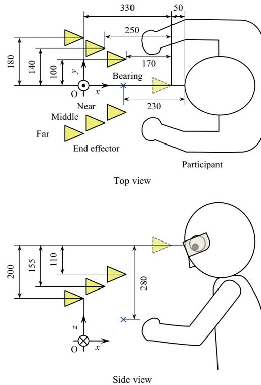
Fig. 1. Schematic diagram of the human-robot interactive locations in psychological experiment (unit: mm)
