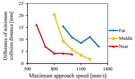
Fig. 9. Effect of avoidance actions: Differences of the minimum collision distances on taking and not taking human avoidance into consideration
