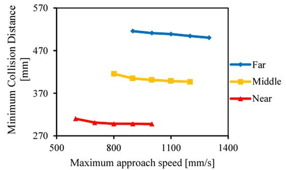
Fig. 8. Relationship between minimum collision distance and maximum approach speed for three conditions (far, middle, near)
