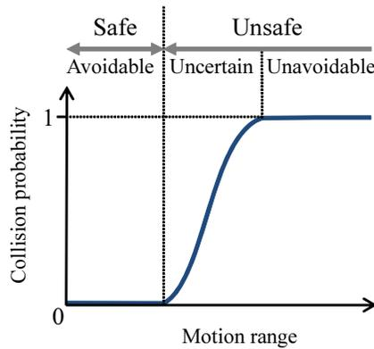
Fig. 7. Safety condition according to collision probability curve
