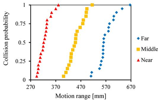
Fig. 6. Collision probability curve for three conditions (far, middle, near) with maximum approach speed set to 1000 mm/s
