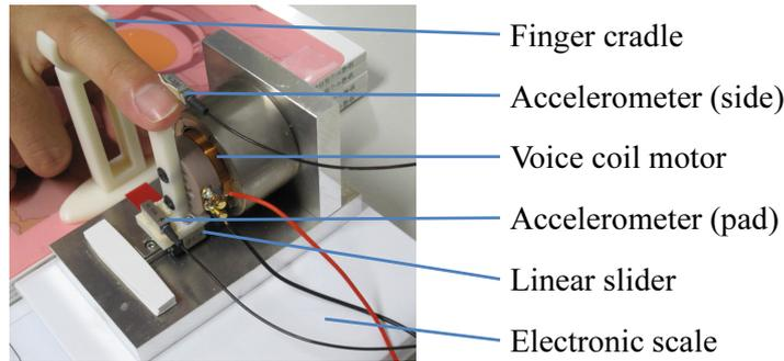
**Fig. 2.** Experimental apparatus for measuring acceleration of a fingertip
