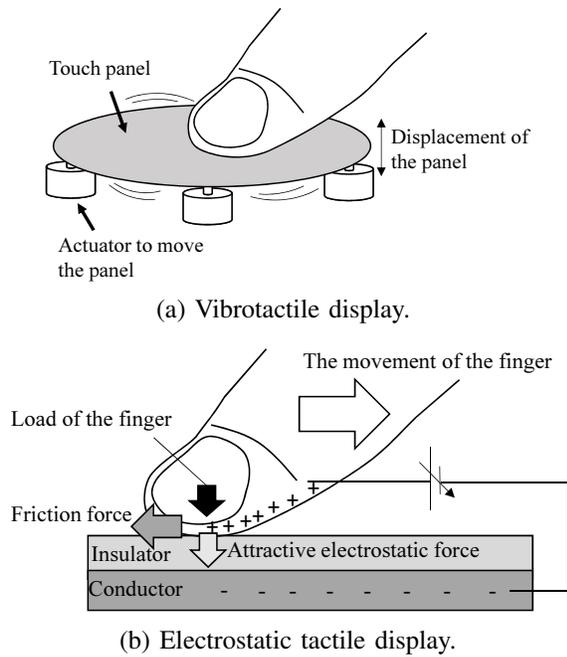
Fig. 1. Principles of vibrotactile and electrostatic tactile displays.
