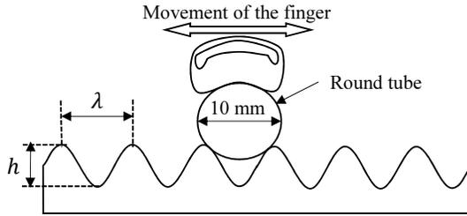
Fig. 3. Sinusoidal grating scale. Participants experienced the grating scale with the round tube.
