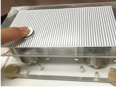
(b) Photograph of the display. A picture of a grating scale is displaced beneath the transparent top panel.
