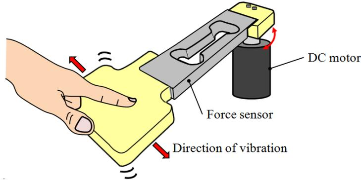
**Fig. 1.** Lateral vibrotactile display based on a DC motor and equipped with a load cell. The finger scans the contactor along the direction of vibration.
