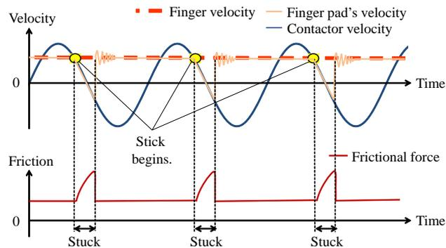
**Fig. 3.** Velocity of the finger and vibrating contactor and the frictional force between them
