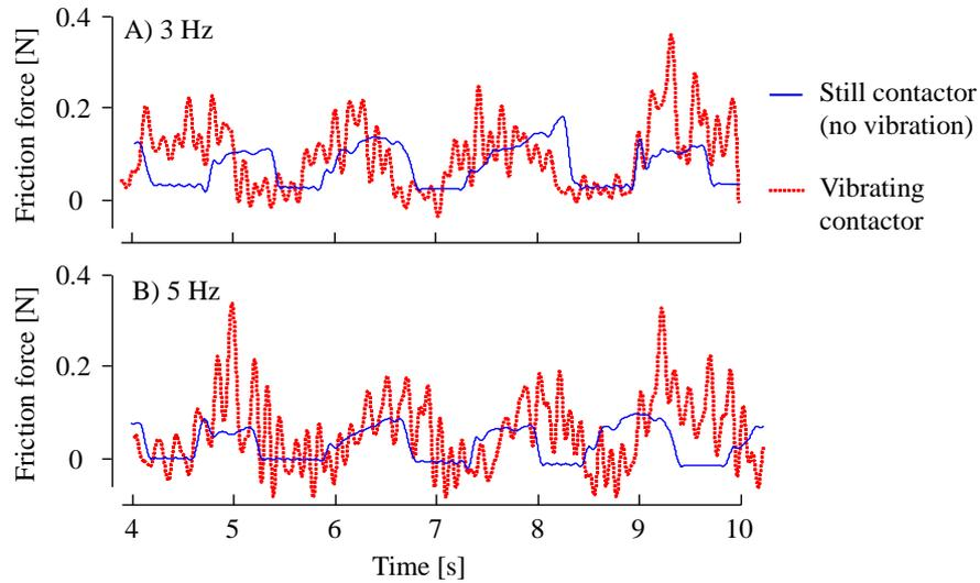
**Fig. 2.** Frictional forces when the finger scanned the contactor with and without vibration (A : 3 Hz, B : 5 Hz). During periods in which the frictional force was nearly zero, the finger was not in contact with the contactor. Sticking was more frequently observed between the vibrating contactor and finger than between the still contactor and finger. For visual clarity, components larger than 10 Hz have been filtered out.
