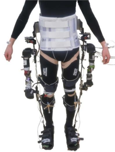
Fig. 2. MALO : Motor Actuated Lower-limb Orthosis
