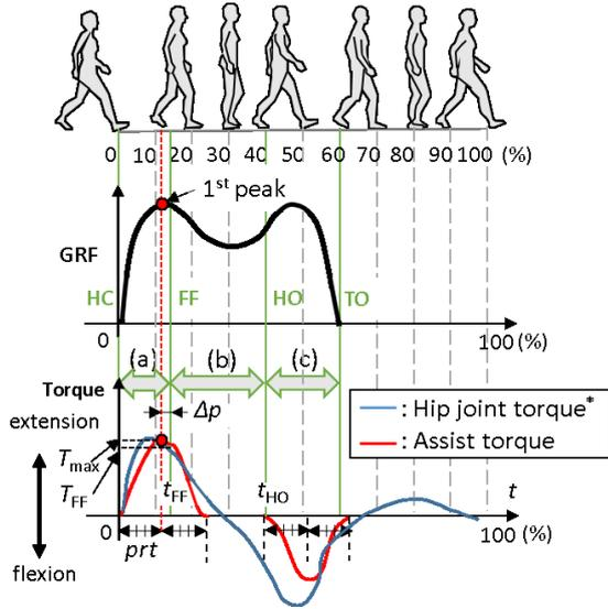
Fig. 1. Pattern of GRF and assist torque applied to hip joint (\* Hip joint torque is cited from Winter DA et.al(1996))
