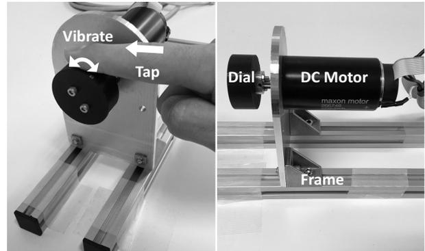
Fig. 1. One degree of freedom force display with direct DC motor drive
