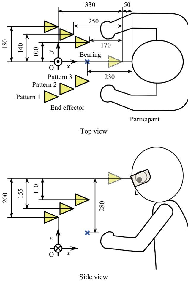
Fig. 4. Schematic diagram of the interactive human-robot locations during the psychological experiment (unit: mm)
