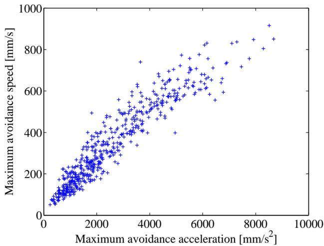
Fig. 7. Relationship between the maximum avoidance acceleration and maximum avoidance speed
