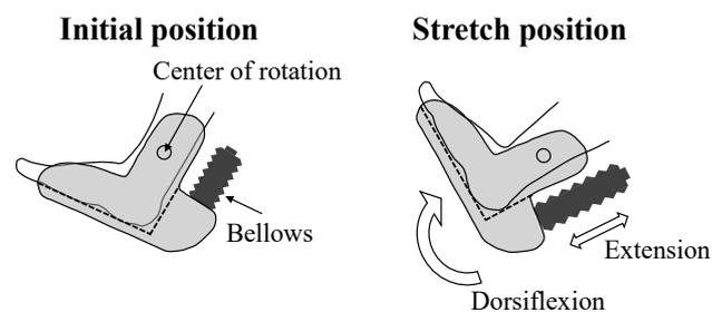
Fig. 1. Operation principle of stretching device.
