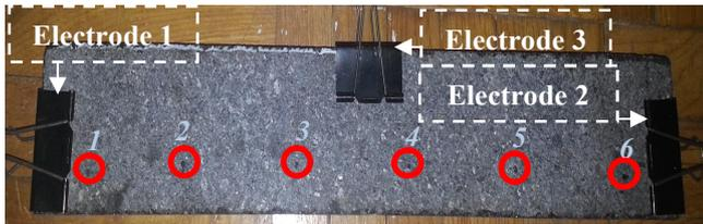
Fig. 2. Granite touch panel used with mounted electrodes.
