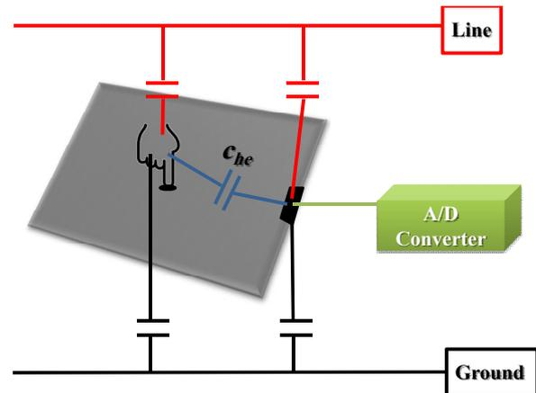
Fig. 1. Concept of the AC hum granite touch panel.
