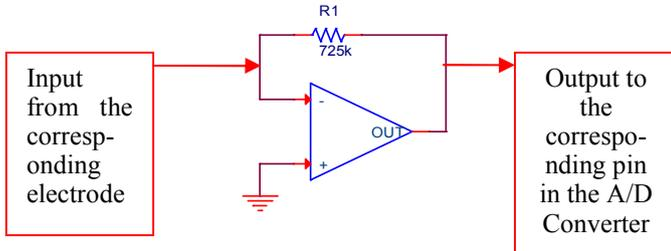
Fig. 3. Current-to-voltage converter circuit schematic.
