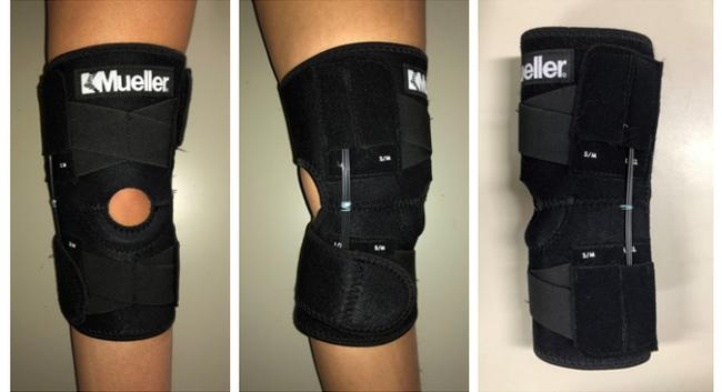
Fig. 2: Knee assistive device built from a commercial knee supporter with shape-memory-alloy wires.
