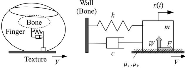
Fig. 7. Single-DOF Vibration Model for Simulating Stick-Slip Motion
