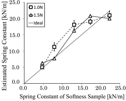
Fig. 5. Validation of Estimation Method for Spring Constants (Error bars for 1.5 N are too small to be seen)
