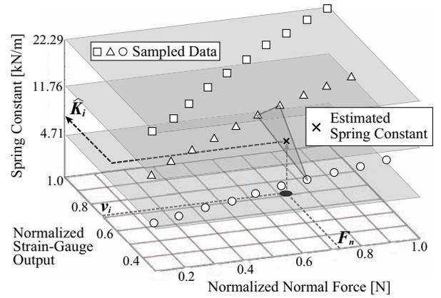
Fig. 4. Mapping Model for Estimating Spring Constants
