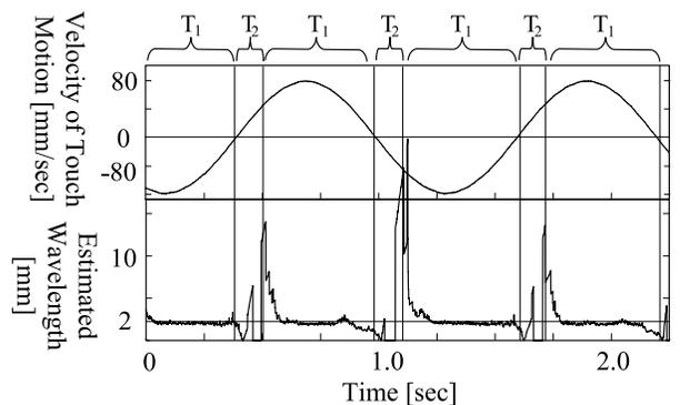
Fig. 7. A transition of the estimated surface wavelength when the sensor scanned the sample at the sinusoidal velocity;  $\lambda = 2$  mm,  $v = 70 \sin(2\pi 0.83t)$  mm/sec
