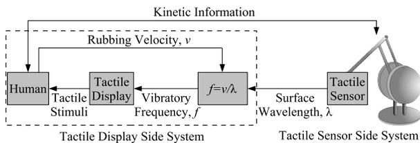
Fig. 1. A block diagram of a master-slave typed roughness feeling telepresence system by surface wavelengths of target objects, which cancels the mismatches between tactile and kinetic sensations of human operators
