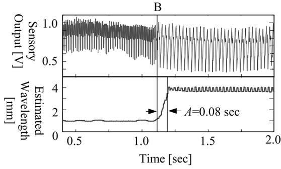
Fig. 8. Example of the sensory outputs and the estimated surface wavelengths when the sensor scanned two different specimens
