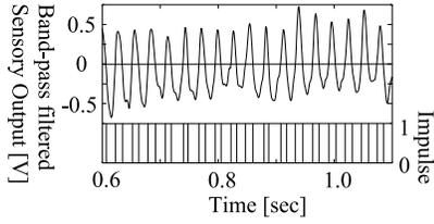
Fig. 4. Example of band-pass filtered sensory outputs and impulses which are emitted at zero crosses
