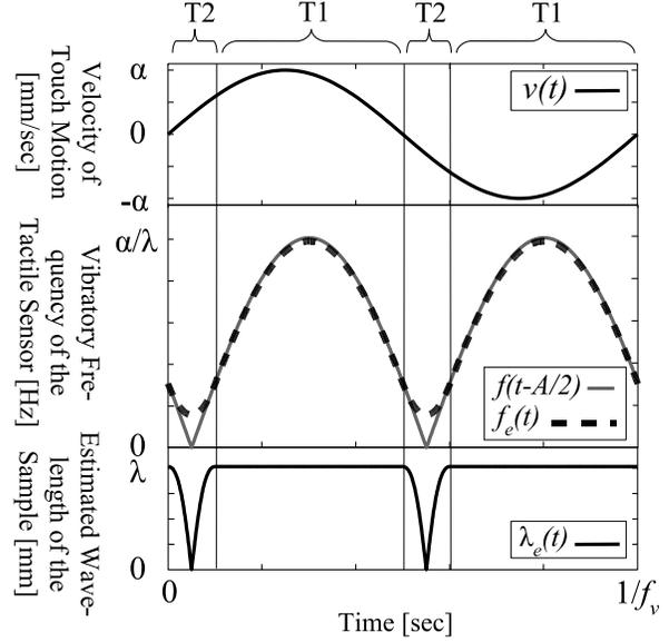
Fig. 5. Examples of simulated values of the rubbing velocity  $v(t)$ , the true and the estimated vibratory frequencies  $f(t - A/2)$ ,  $f_e(t)$  and the estimated wavelength  $\lambda_e(t)$ :  $A = 0.2$  sec,  $\lambda = 2.0$  mm,  $\alpha = 100.0$  mm/sec,  $f_v = 1.0$  Hz,  $X = 0$  mm
