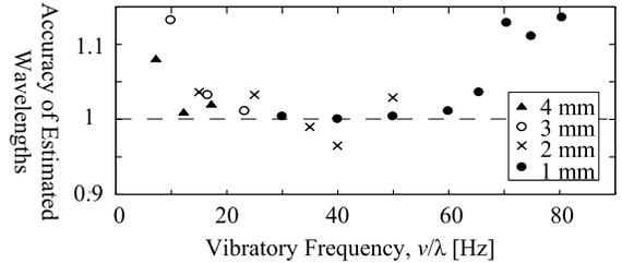
Fig. 6. Accuracy of wavelength estimation when samples were scanned at constant speeds
